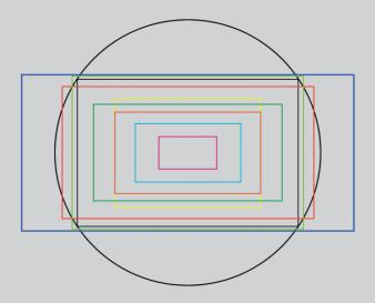
ARRI Alexa65 (54.12x25.59 mm), ø 60.0 mm RED Weapon 8K (40.96x21.6 mm), ø 46.3 mm ARRI Alexa 65 Vista Vision (37.7x25.5 mm), ø 45.0 mm Full Frame Stills (36x24 mm), ø 43.3 mm RED Dragon 6K Full Frame (30.7x15.8 mm), ø 34.5 mm ARRI Alexa 4x3 (23.8x17.8 mm), 29.7 mm ARRI Alexa 16x9 (23.8x13.4 mm), ø 27.3 mm GH4 16x9 (17.3x9.7 mm), ø 19.8 mm 2/3" (9.6x5.4 mm), ø 11.0 mm
